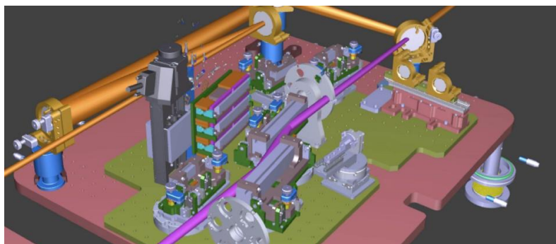
Figure 1: Drawing of the optomechanics mounted on the SE10 beamline for XUV/IR pulses recombination. It implements a monochromator and spectral selection by reflexion on multilayer coatings.
